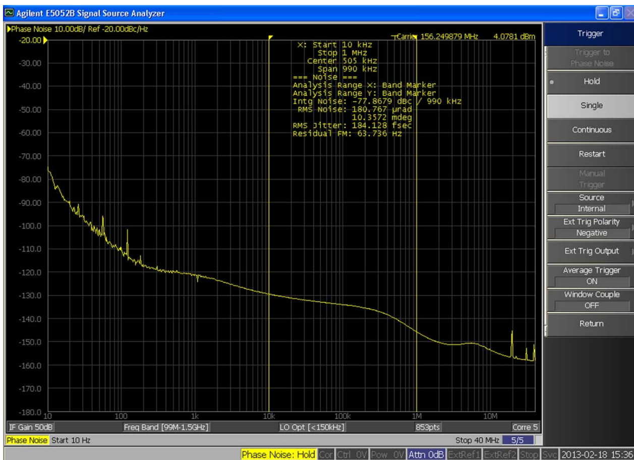
Figure 1. Si535/536 Typical Phase Noise at 156.25 MHz
